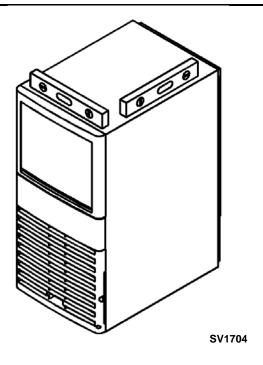
**Checking Ice Machine Level**
